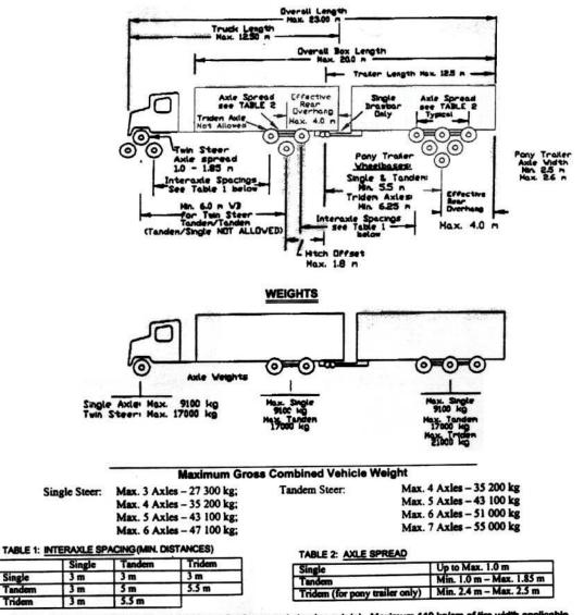
Maximum 3 000 kg/tire applicable to all axles except steering axle(s). Maximum 110 kg/cm of tire width applicable to all tires. Effective January 1, 2005, 100 kg/cm of tire width applicable to all tires. Notes:
